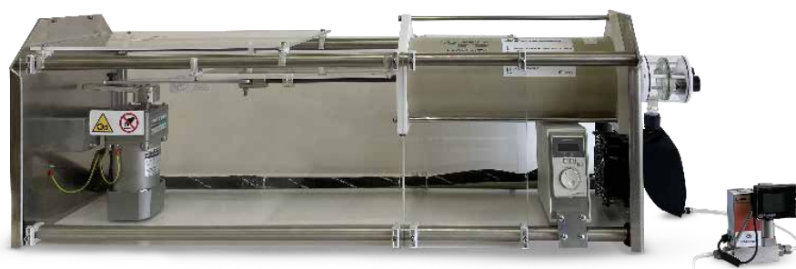
COSMED Metabolic Simulator is an advanced verification tool to simulate human subject gas exchange and respiratory pattern for both clinical and research settings
