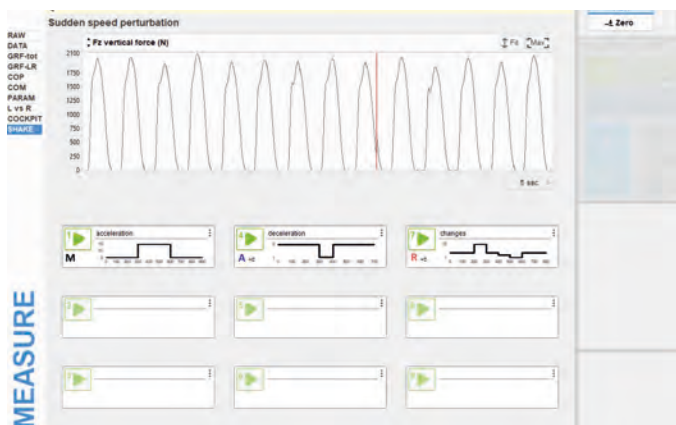
The perturbation mode will allow sudden speed changes to simulate slips and trips on h/p/cosmos treadmills with UserTerminal Touch (Pro).
