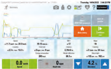
The UserTerminal touch summary screen shows all relevant data of the workout including average and max. speed, elevation, duration and heart rate as well as biomechanical indicators as step lengths and cadence.
