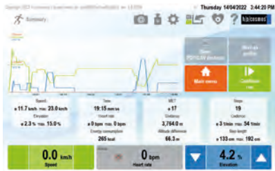
The UserTerminal Touch summary screen shows all relevant data of the workout including average and max. speed, elevation, duration and heart rate as well as biomechanical indicators as steplengths and cadence.
